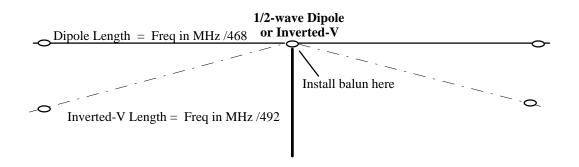
The key to success when operating low-power SSB is a properly-installed full-sized resonant antenna. Dipoles and inverted-Vs generally work best for regional coverage.
