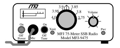
**Receiving:** The MFJ-9475 is extremely simple to operate. To get started, press the *POWER* switch on (the green *PWR* LED should illuminate). Adjust the *VOLUME* control for a comfortable listening level. Now, tune in your station with the *VFO TUNING* knob. That's all there is to it!
